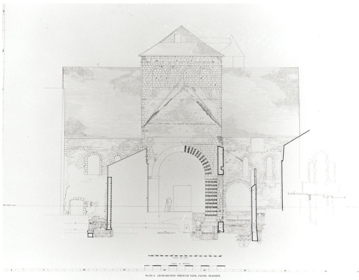
Abbatiale, coupe transversale nef côté transept, 1953. Dessin, in : FORSYTH, George H, The church of St. Martin at Angers, Princeton, University Press, 1953, planche VI.
